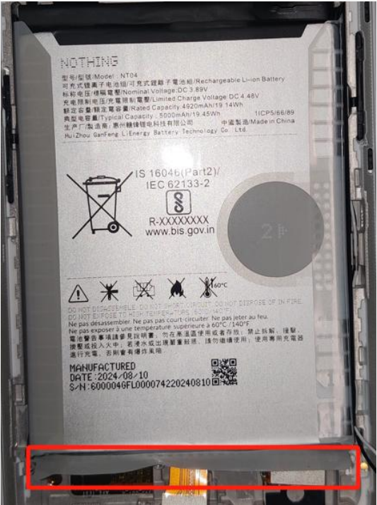
a). Gently tear off the easy-tear paper on the surface of the battery, refer to position 1
