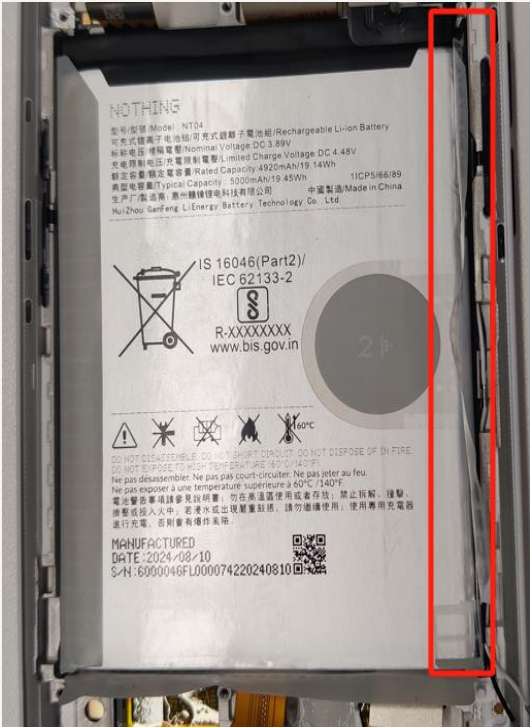
b). Gently tear off the easy-tear paper on the surface of the battery, refer to position 2
