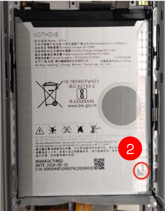
b). Gently tear off the easy-tear paper on the surface of the battery, refer to position 2
