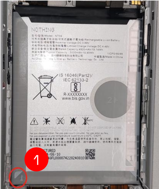
a). Gently tear off the easy-tear paper on the surface of the battery, refer to position 1
